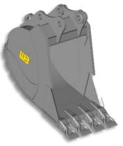
**METRO STYLE BUCKETS** are to be used in low-impact materials such as dirt and loam where one wants to leave a smooth floor and minimal spillage. This bucket is engineered specifically for spade (wide tip) teeth, and where end shanks are set straight to create smooth edge; ideal for pipe and/or tile work.
