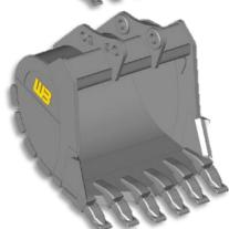
**HEAVY PENETRATION BUCKETS** are used in heavy abrasive applications where breakout force & cycle times are important. Breakout force is maximized due to decreased tip radius and increased pin spread. In addition, Heavy Penetration Rock Chisel Teeth would be installed where applicable.
