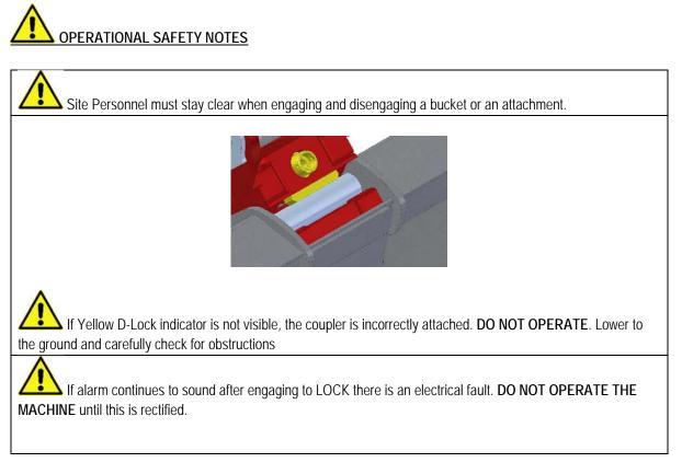
Due to the self-tightening and automatic wear compensation features of this coupler it is recommended that the locking cylinder be disengaged at the end of each day.
