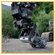
**High Flow Swivel** For attachments with high oil flow.
