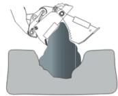
**BOTTOM DUMPING**Ideal for trench filling or dumping into a container.
