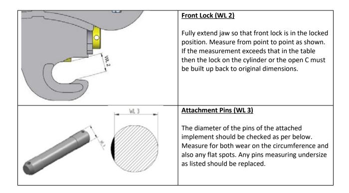
OEM mounting pin diameters should be checked against the supplier's recommendations. Replace pins if required.
