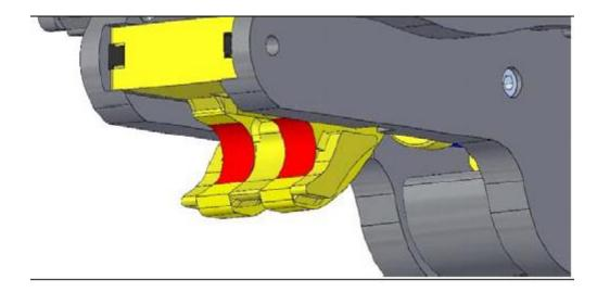
There are three wear areas that could be causing contact. It may be one area that is worn excessively or any combination of all three areas. All three areas should be checked and rectified if the below wear limits are exceeded.
