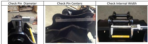
Note, Internal width should not exceed the width of the coupler more than 4mm per side, If coupler is used on Under cutters, rock saws or any other attachment which has a significant side load, the coupler MUST be a tight fit.
