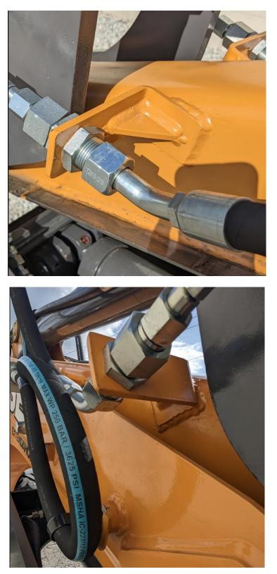
P-CLAMP HOSE RETAINER, ONE ON EACH SIDE: (see "auxiliary extension kit" detail on following pages)
