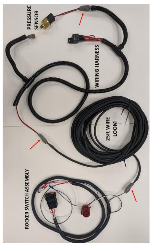
Wiring Harness / Wiring Loom / Rocker Switch / Pressure Sensor
