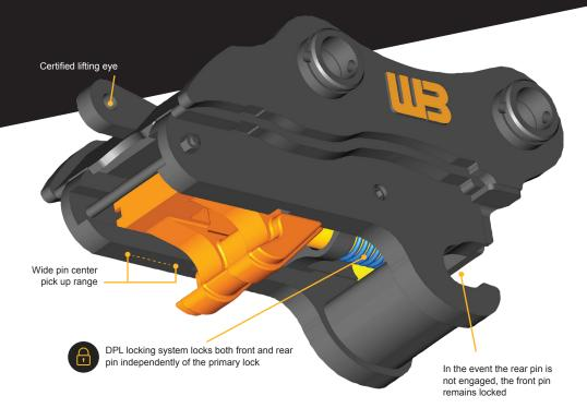
The simple, easily serviceable design of the D-Lock combined with world leading safety features makes the D-Lock the safest coupler on the market today. The D-Lock Coupler is dual locking, meaning attachments remain securely engaged on both pins in the event of loss of engagement force.
