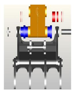
2. When centralized, measure the gap remaining on either side to determine the best combination of shims to use.
