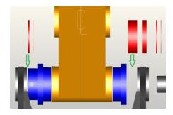
3. Install selected shims while inserting pivot pin (one side at a time)
